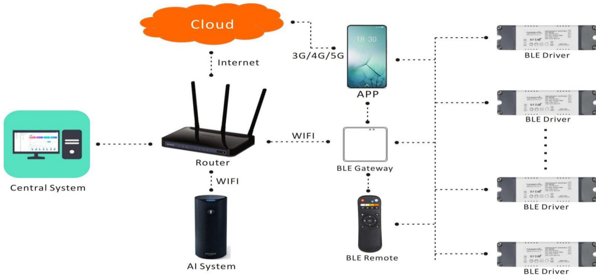
BLE Sigmesh Smart Lighting System
